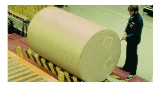
The stripping assist has a central function in the roll transport. In addition to the actual stripping this position is also ideally suited for pasting preparation, checking the roll condition, barcode input, checking the roll gross and net weight plus the perfect alignment of the roll for the following automatic processes.
