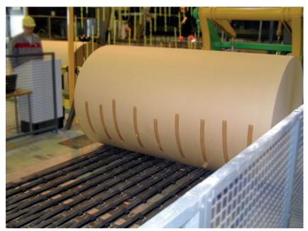
MoveRoll conveyors have high handling capacity and can be used with all different roll sizes
